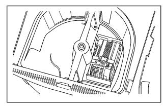
Locate the tire sealant and compressor kit on the driver side of the vehicle, near the back corner of the trunk.
